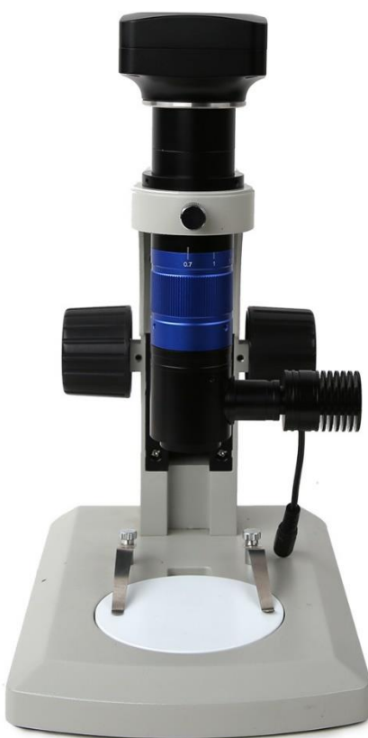
BS-1008-W100-TV050+BS-1008CL+BS-1008SL(Coaxial Light Module)+ USB CMOS Camera
