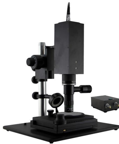
BS-1080FC with pole column stand (coarse&fine focus), X-Y stage, coaxial illumination and LED ring light, Plan APO metallurgical objective
