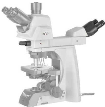
2 Viewing heads (Face to Face)
