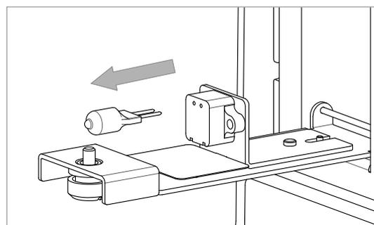
8.3.6. Hold a new bulb with silk cloth to avoid fingerprint and dust affect bulb brightness and service life (Fig.8-6), and insert the bulb holder. (Fig.8-5 in opposite direction)
