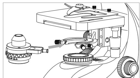
When installing independent condenser, please turn mark **TOP** upwards.
