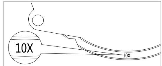
Putting phase contrast objective in the light path, rotating phase contrast condenser turnplate, relevant multiplying power scale in front side (Fig.5-14), when feeling phase contrast slider in right location, can begin phase contrast observation.
