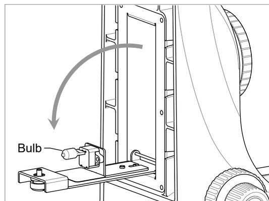
8.3.5. Please be sure that the bulb is cool, pull out the broken bulb. (In direction Fig.8-5)
