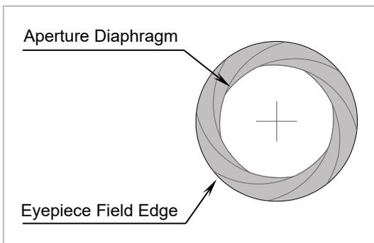
Step 6. Adjustment of field diaphragm and centering
