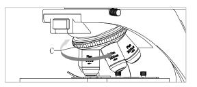
Putting 10X objective in the optical path by rotating condenser C (Fig. 4-4), observing in right eyepiece, adjusting coarse focusing knob(O,V) (Fig. 4-5) to get outline image, then slowly rotating fine focusing knob ( $\mathbf{N}$  or  $\mathbf{W}$ ) until getting more clearer image.
