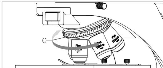
Putting 10X objective in the optical path by rotating condenser C (Fig. 4-4), observing in right eyepiece, adjusting coarse focusing knob(O,V) (Fig. 4-5) to get outline image, then slowly rotating fine focusing knob (N or W) until getting more clearer image.
