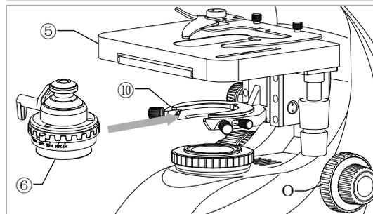
(Fig. 3-11) Loosening screw for condenser (J) (not unscrew completely), inserting condenser ⑥ to the holder and tighten up (J). Rotate adjusting knob for condenser (Q) to the highest position.
