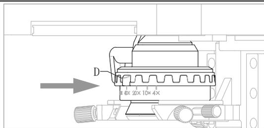
(Fig.4-10) Compared with Abbe condenser, using swing-out condenser can make objective aperture diaphragm match with illuminating system aperture diaphragm. Upper condenser must be moved out of light path in 4X or 10X objective, if in high power objective, should adjust upper condenser in light path.
