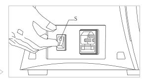
(Fig.4-2) Turn on power switch (S) and change to position (I). Rotate Brightness adjusting knob (M) for eyepiece field brightness.
