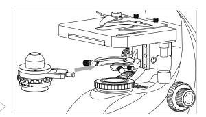
When installing independent condenser, please turn mark **TOP** upwards.
