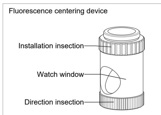
7.5.1 Holding the installation insection (Fig.7-14) and installing it on the nosepiece, turning the cover of centering device to align the observation window.
