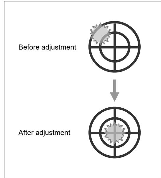
7.5.5 Rotating adjusting knob F28 and F29 which on the mercury lamphouse, light source will move to the cross target line centre. (Fig.7-15)
