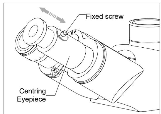
sliter clear imaging, then locking the screw. (Fig. 5-15)
