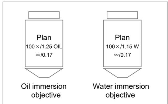
At this time, condenser should be gently rotated back and forth several times, making specimens of relative movement to the objective, to eliminate air bubbles in the oil, avoid bubble influence for image.
