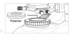
Take out the accessory module box(2) from the stand and put in analyzer (Fig. 5-3), the putting back accessory box following Step 3. (Fig 3-8)
