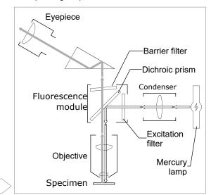
The device consisting of reflecting fluorescence illuminator, mercury lamp power box and fluorescence objectives are combined with mainbody to make up fluorescence microscope. The device is designed and manufactured with Epi-excitation principle and provided with 4 group excitation filters system of FL4: blue (B), green (G), violet (V) and ultraviolet (UV). Auramine is optional used for tuberculosis 455mm.
