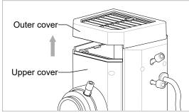
8.4.4 Reconfirm mercury lamp and relevant device are complete are cooling, loosening the two fixed screw. (Fig. 8-9)
