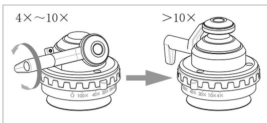
(Fig.4-11) Sample contrast is generally low, so condenser aperture diaphragm must be set from 70% to 80% of numerical aperture, also can observe in eyepiece tube and adjust the microscope without eyepiece.
