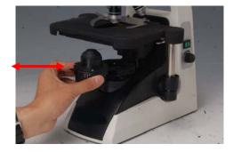
the label in the condenser forward and move the condenser into the bracket. At last tighten the screw.
