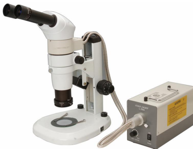
BS-3060 with coaxial episcopic illuminator
