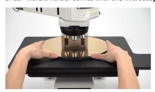
12" wafer and smaller size wafer can be observed with this microscope, with fast and fine movement stage handle, it can greatly improve the working efficiency.
