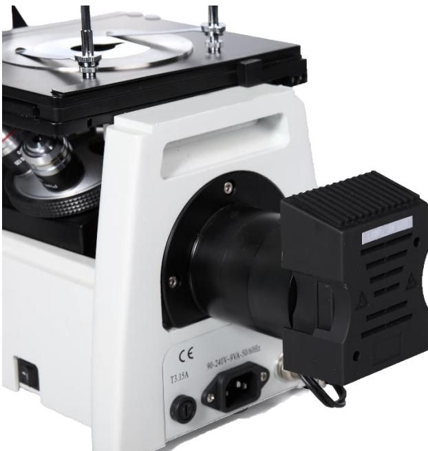
3. Reflected Koehler illumination system with iris diaphragm and centerable field diaphragm, wide range voltage 90-240V, 6V/30W high brightness halogen bulb and long working life LED bulb(optional).
