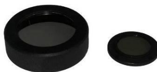
Simple polarizing unit Polarizer & analyzer
